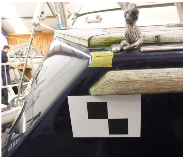
Examples of forward and aft freeboard points as being at the top point at a tangent at 45 degrees with checkerboard set up below. The vertical distance from the center of the checkerboard to the freeboard point needs to be measured separately
